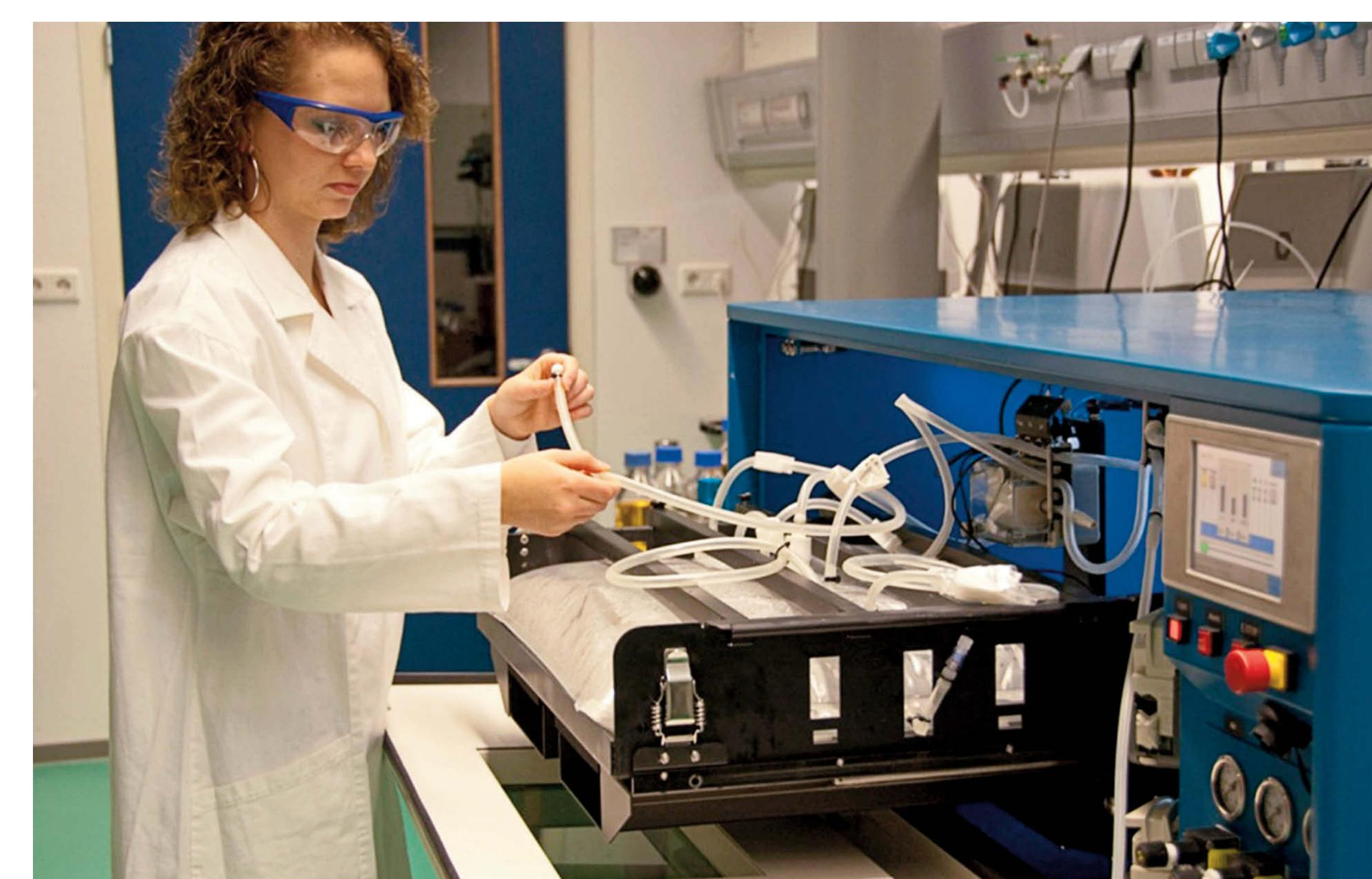
The PID algorithm in the control strategy was applied to the key parameters pH, DO, glucose and Temperature.
